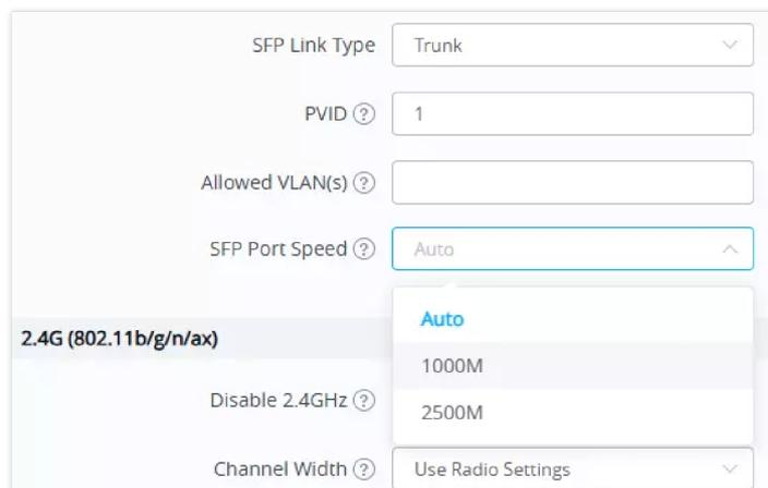
A detailed view of the configuration for SFP Link Type. The SFP Link Type is set to Trunk, PVID is 1, Allowed VLAN(s) is empty, SFP Port Speed is Auto, and Channel Width is Use Radio Settings. A dropdown menu for SFP Port Speed is open, showing options: Auto (highlighted), 1000M, and 2500M. The 2.4G (802.11b/g/n/ax) section is also visible.
