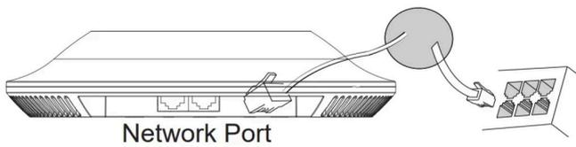
RJ45 Ethernet Cable to power over Ethernet (PoE+) Switch.
