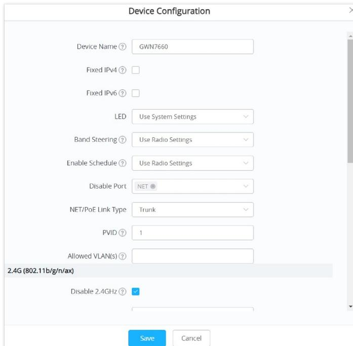
A "Device Configuration" dialog box for device GWN7660. It contains several configuration fields: Device Name (GWN7660), Fixed IPv4 (checkbox), Fixed IPv6 (checkbox), LED (Use System Settings), Band Steering (Use Radio Settings), Enable Schedule (Use Radio Settings), Disable Port (NET), NET/PoE Link Type (Trunk), PVID (1), Allowed VLAN(s) (empty), and a section for 2.4G (802.11b/g/n/ax) with a checked "Disable 2.4GHz" checkbox. "Save" and "Cancel" buttons are at the bottom.
