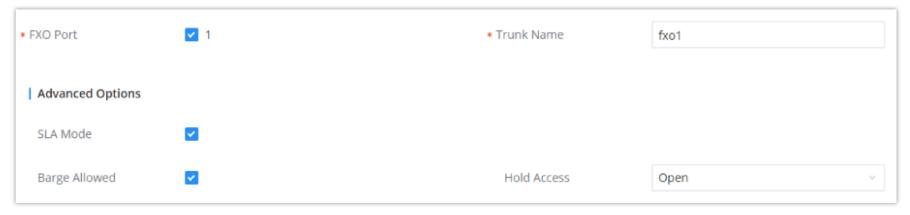
Enable SLA Mode for Analog Trunk
