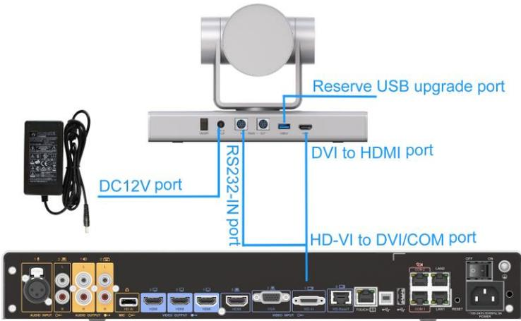
Use an HD-VI adapter if the Box 500's HDMI input is used for the demo and no HDMI port is available for direct connection with the camera. Insert the supplied HD-VI to DVI/COM adapter into the Box 500's HD-VI port. Connect it to the DVI-HDMI adapter (not included) and to the Camera 200's HDMI port, and then connect the COM cable to the Camera 200's RS232-IN port.
