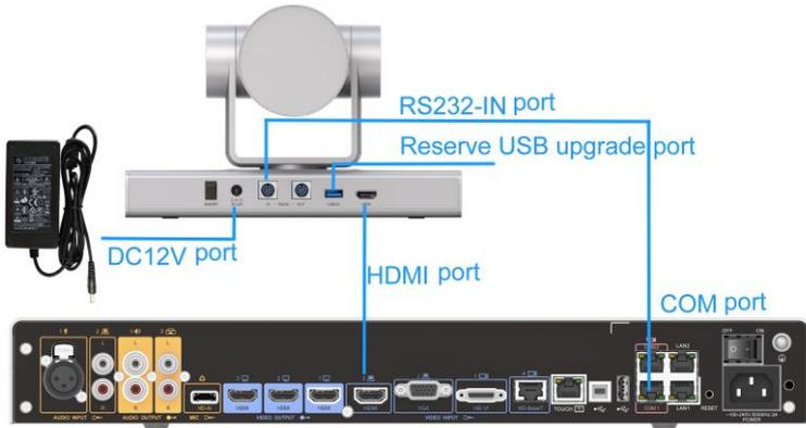
If the Box 500's VGA port is used for input in the demo or multiple HDMI input ports are available, connect the HDMI video input port of the Box 500 to the camera's HDMI port, and the Box 500's COM1 to the camera's RS232-IN port. Suggestion: Reserve a plugged-in USB cable for seamless PC upgrades in the future.
