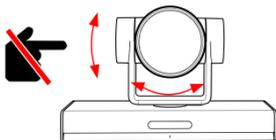
Do not manually rotate or stop the camera from rotating when it is operating properly. Otherwise, the camera must be restarted.
