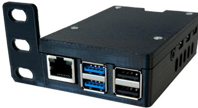
1. Connect the device to your home / business network with an Ethernet cable to the RJ45 port
