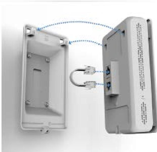
4. Secure e430 to the bracket using Torx (or standard) screw on the lower edge of e430.
