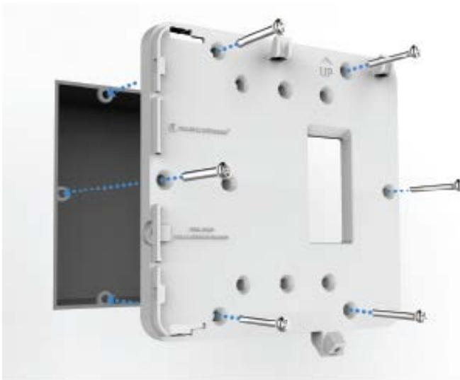
2. Place Cambium dual-gang wall bracket on the gang box and secure with at least two screws.
