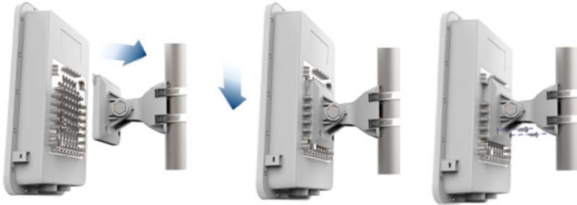
4. Insert RJ45 to radio housing and the lock cable gland to radio housing with 1.5Nm to 2Nm torque.
