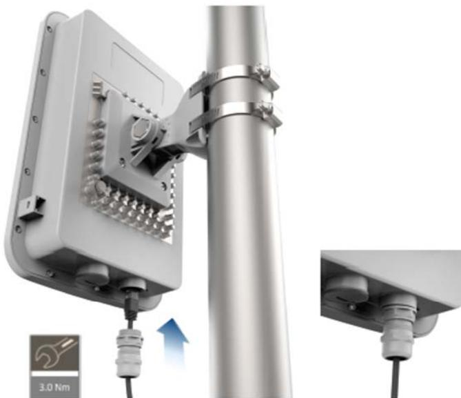
5. Align Radio to required angle by tilting up and down. The maximum radio tilting angle is  $\pm 40^\circ$ , with an incremental of  $10^\circ$ .
