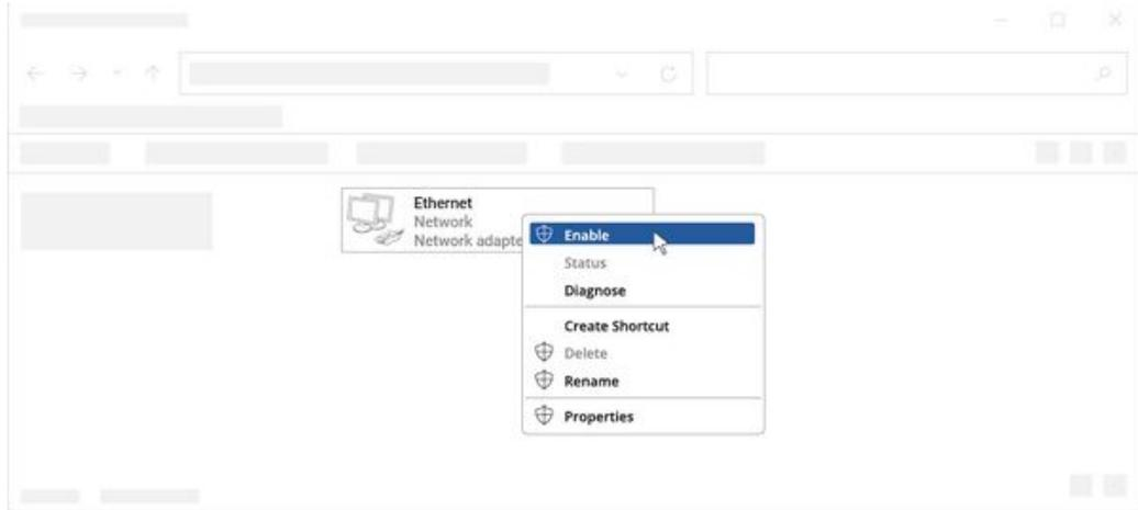
2. Check if IP and DNS are obtained automatically. Right-click on Network Adapter and select Properties. Then select **Internet Protocol Version 4** and click Properties.
