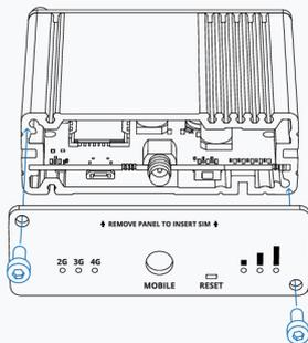
4. Attach the Mobile antenna to the connector labeled "MOBILE".
