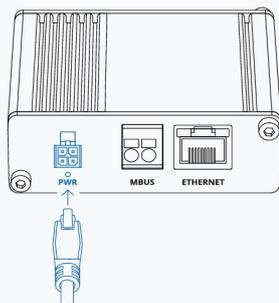
6. Connect to the device with an Ethernet cable connected to the LAN port.
