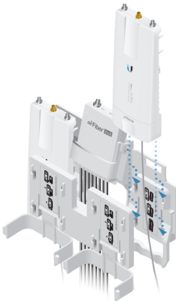
5. Mount the airFiber 5X radios to the *8x8 Radio Bracket*:
