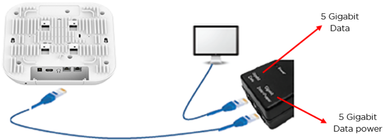
Figure 2 : Installation of Enterprise Wi-Fi AP to PoE adapter
