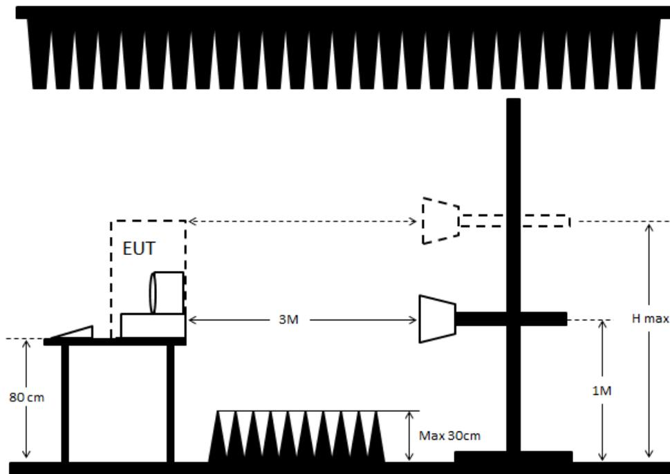
Remark : When EUT height is over 172cm , H max = Top of EUT
