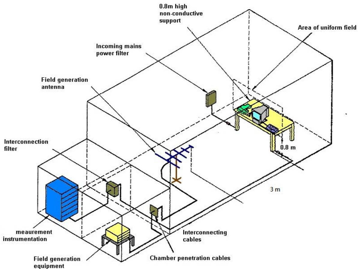
The procedure defined in this part requires the generation of electromagnetic fields within which the test sample is placed and its operation observed. To generate fields that are useful for simulation of actual (field) conditions may require significant antenna drive power and the resultant high field strength levels.
